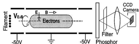
FIG. 1. The cylindrical experimental apparatus with phosphor screen/CCD camera diagnostic.
