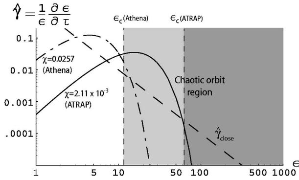
FIG. 3. The rate  $\hat{\gamma}$  at which energy is lost from the bound charge system due to mobility drag (for Athena and ATRAP parameters); and for Glinsky–O’Neil small impact parameter collisions (dashed line). Drag dominates over a finite range in binding energy, depending on the factor  $\chi$ .
