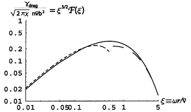
FIG. 2. The normalized recombination rate  $\gamma_{\text{drag}} / \sqrt{2\pi\chi} n \bar{v} b^2 = \xi^{3/2} \mathcal{F}(\xi)$  due to distant collisions (solid line) plotted against the adiabaticity parameter  $\xi = \omega r / \bar{v}$ . We have assumed  $\omega = ec / Br^3$ . The limiting forms for  $\xi \ll 1$  (dotted line) and  $\xi \gg 1$  (dashed line) are also shown. The drop in  $\gamma$  at high  $\xi$  comprises the adiabatic cutoff.
