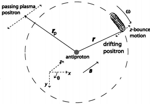
FIG. 1. A guiding center atom. The positron  $\mathbf{E} \times \mathbf{B}$  drifts in the electric field of a stationary antiproton while oscillating back and forth along the magnetic field in the potential well of the antiproton. The drift orbit frequency  $\omega \approx ec/Br^3$  for small bounce motion and is slower than oscillations parallel to the field.
