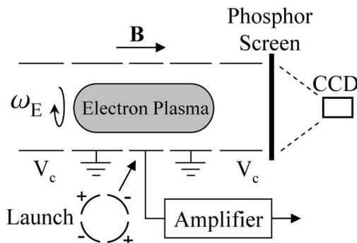
FIG. 1. Electron trap with CCD camera density diagnostic. The wall signal from sector electrodes is used to measure the wave amplitudes.
