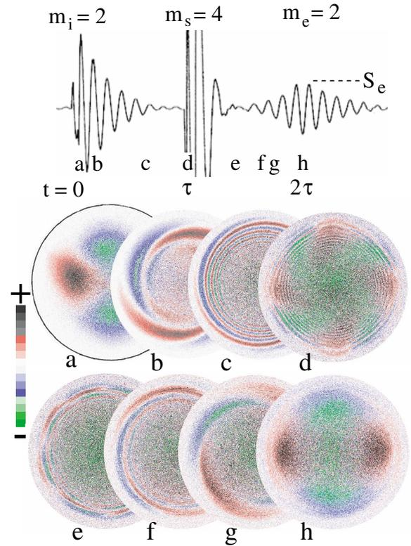
FIG. 2 (color). The top image shows the measured wall signal; below are experimental density perturbation images at eight successive times, corresponding to the times marked in the top trace.
