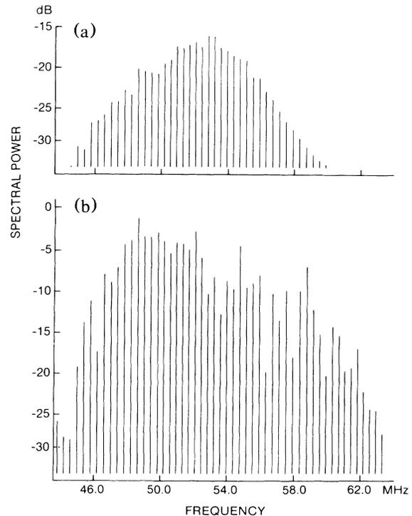
FIG. 2. (a) Spectrum launched by the arbitrary wave-form generator. The spectral lines shown here [and in Figs. 3(b) and 4(a)] are meant to show only the measured power at each mode frequency. The finite linewidth at each frequency has been suppressed for clarity. (b) Spectrum downstream.  $V_b = 60.0 \text{ V}$ ,  $I_b = 140 \mu\text{A}$ ,  $V_s = 2.5 \text{ kV}$ ,  $\eta_p = 0.098$ , and  $\eta_s = 0.36$ .
