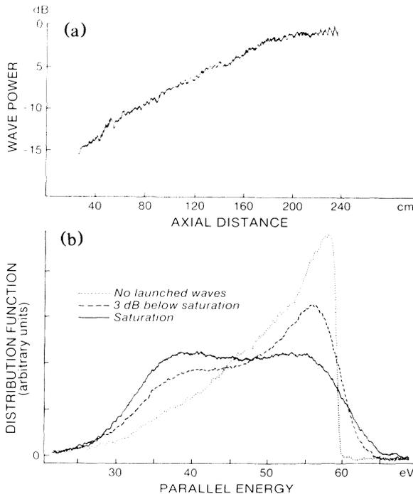
FIG. 1. (a) Total wave power vs axial distance. Beam voltage is  $V_b = 60.0 \text{ V}$ , beam current is  $I_b = 110 \mu\text{A}$ , and spreader bias voltage is  $V_s = 2.0 \text{ kV}$ .  $\eta_p = 0.065$  and  $\eta_s = 0.17$ . (b) Time-averaged beam parallel-energy distribution function at various positions vs parallel energy. Same parameters as (a). The launch level is held constant.
