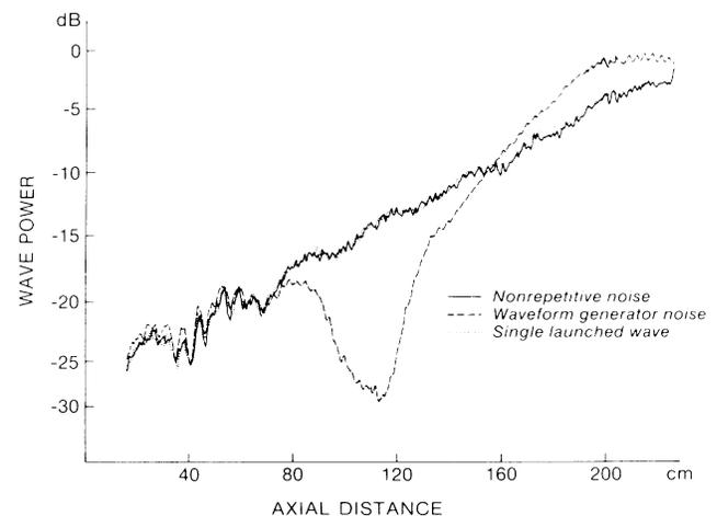
FIG. 4. Wave power vs axial distance for various launched signals: Repetitive noise (dashed curve), nonrepetitive noise (solid curve), and a single wave (dotted curve).  $V_b = 60.0$ ,  $I_b = 140 \mu\text{A}$ ,  $V_s = 2.5$  kV, and  $f = 62.34$  MHz.  $\eta_p = 0.055$  and  $\eta_s = 0.19$ .
