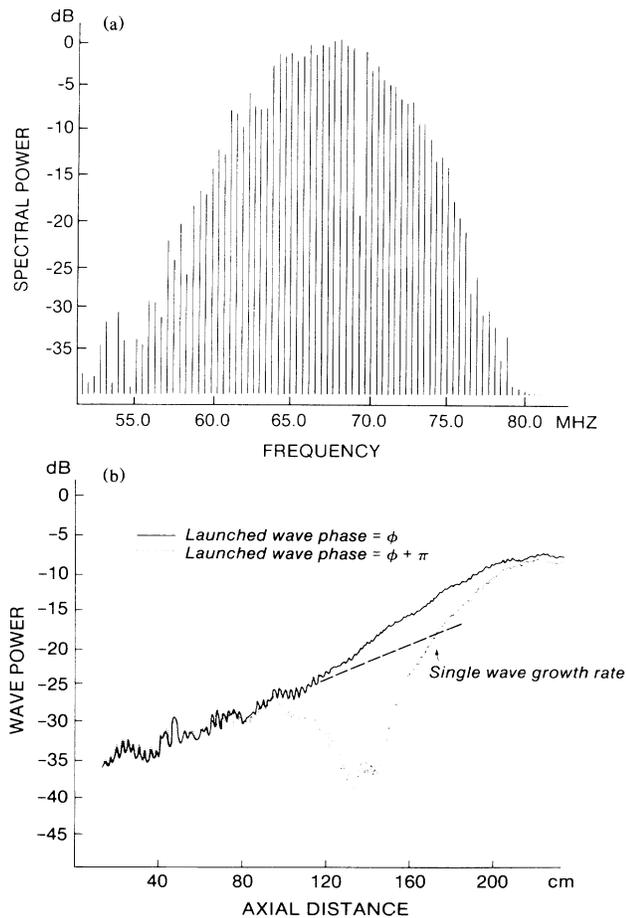
FIG. 3. (a) Spectrum used to further investigate the mode coupling. (b) Wave power vs axial distance of a mode with phase equal to  $\phi$  (solid curve) and of the mode with phase equal to  $\phi + \pi$  (dotted curve).  $V_b = 60.0$ ,  $I_b = 110 \mu\text{A}$ ,  $V_s = 2.0$  kV, frequency,  $f = 69.12$  MHz.  $\eta_p = 0.038$  and  $\eta_s = 0.20$ .
