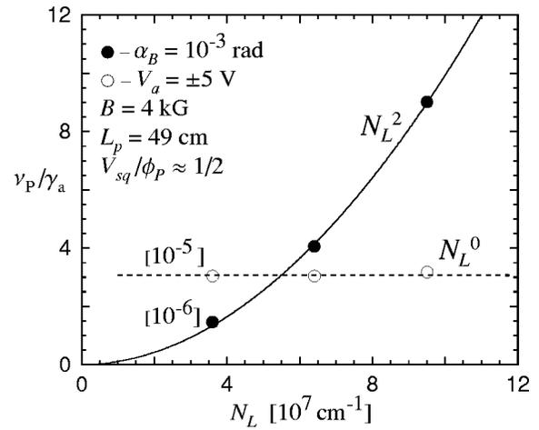
FIG. 9. Normalized transport rate  $\nu_p/\gamma_a$  at constant fraction of trapped particles ( $V_{sq}/\phi_p$ ) vs plasma line density  $N_L$  for magnetic and electric asymmetries.
