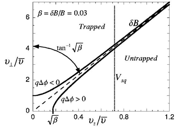
FIG. 12. Velocity-space separatrices for magnetostatic and/or electrostatic trapping.
