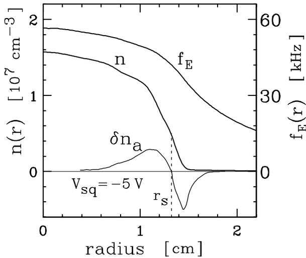
FIG. 2. Radial profiles of density  $n(r)$ ,  $\mathbf{E} \times \mathbf{B}$  rotation frequency  $f_E(r)$ , and measured asymmetry mode eigenfunction  $\delta n_a(r)$ .
