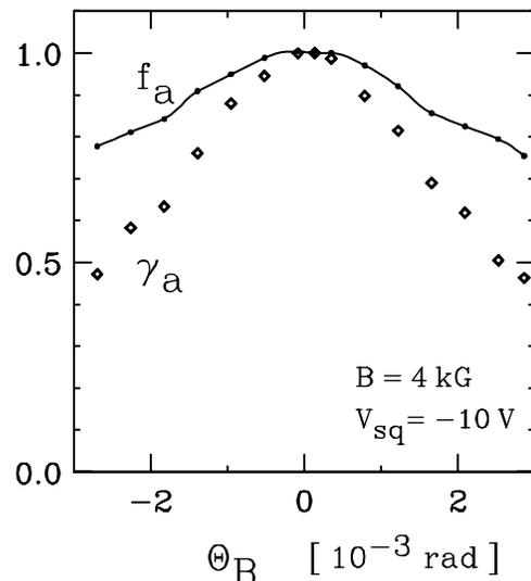
FIG. 5. Measured frequency  $f_a$  and decay rate  $\gamma_a$  vs magnetic tilt  $\theta_B$ , normalized to values at  $\theta_B = 0$ .
