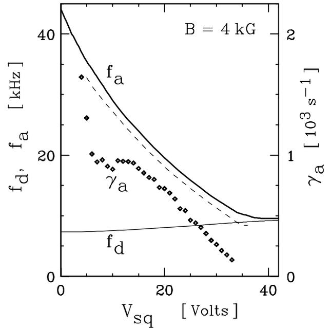
FIG. 3. Measured frequencies  $f_a$  and  $f_d$  and decay rate  $\gamma_a$  vs squeeze voltage  $V_{sq}$ , and  $f_a$  calculated from the kinetic model (dashed line).
