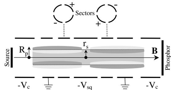
FIG. 1. Schematic of the cylindrical trap and squeezed electron column with asymmetry mode, showing the positive and negative trapped and untrapped density perturbations.
