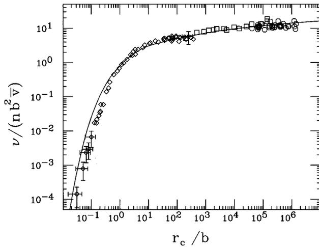
FIG. 1. Normalized relaxation rate [ $\nu/(nb^2 \bar{v})$ ] vs. cyclotron radius divided by distance of closed approach ( $r_c/b$ ). The diamond points  $\diamond$  were obtained using the balanced heating technique, square points  $\square$  were obtained using the unbalanced technique, and the circular points  $\circ$  are data obtained by Hyatt, Driscoll and Malmberg. The solid curve is the Glinisky *et al.* Monte Carlo prediction.
