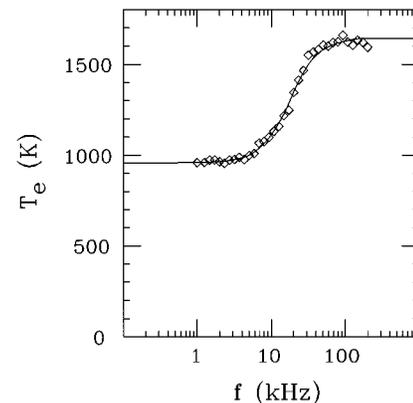
FIG. 6. Plasma temperature after heating  $T_e$  vs. compression frequency  $f$ . Heating for a fixed time,  $t_h = 4$  ms. The points are experimental data and the solid curve is a prediction of the model.
