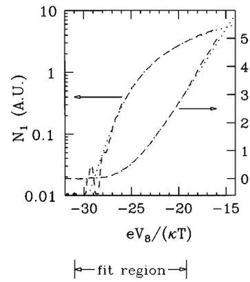
FIG. 11. Normalized number of escaped electrons  $N_1$  vs.  $eV_3/(\kappa T)$  taken for the low temperature analysis, displayed on logarithmic (left) and linear (right) axis. The dash curves are the measured  $N_1$  and the dot curves are the fitted  $C_0 I N_{\text{model}}$ .
