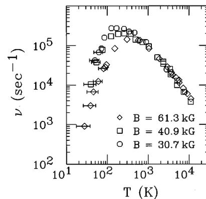
FIG. 9. Measured relaxation rate  $\nu$  vs. temperature  $T$  for various magnetic fields. The plasma density for this data was approximately  $8 \times 10^8$  cm<sup>-3</sup>.
