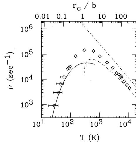
FIG. 8. Measured relaxation rate  $\nu$  vs. temperature  $T$  and  $r_c/b$  for a magnetic field of 61.3 kG. The solid curve is the O'Neil-Hjorth prediction. The dashed curve is the modified Ichimaru-Rosenbluth prediction and the dot-dashed curve is the unmodified Ichimaru-Rosenbluth prediction.
