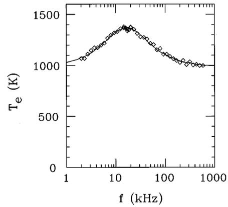
FIG. 5. Plasma temperature after heating  $T_e$  vs. compression frequency  $f$ . Heating comprised of  $H = 80$  contiguous cycles. The points are experimental data and the solid curve is a prediction of the model.
