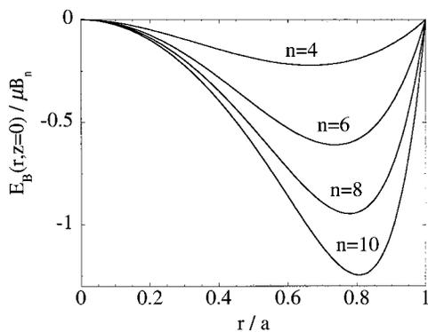
FIG. 8. Boltzmann potential vs radius  $r$  in the  $z=0$  plane for several perfect multipole fields,  $n=4, 6, 8,$  and  $10$ . The potential is shown for the case of maximum well depth, where scaled rotation frequency  $\alpha=\alpha_{\max}$ , so that  $E_B=0$  at  $r=a$ .
