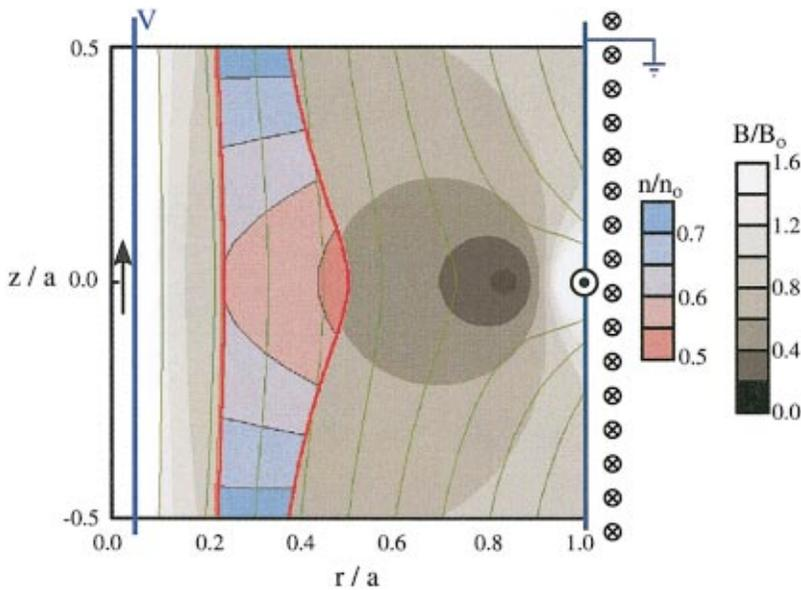
FIG. 5. (Color) An example of plasma confinement in the cylindrically symmetric minimum- $B$  Penning trap. Plasma density is shown by colored contours, magnetic field intensity is shown by gray scale contours. Green lines are magnetic flux surfaces. Arrows denote the location of current-carrying wires. Thick blue lines are electrodes. In this example,  $B_0/B_0 = 2.6$ ,  $B_\theta/B_0 = 0.125$ , and  $V = 0.38\pi en_0 a^2$ .
