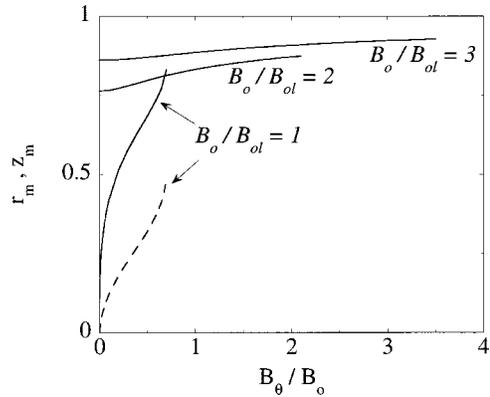
FIG. 4. Location of magnetic minimum versus azimuthal field  $B_\theta$  for three values of the ratio of solenoidal to loop fields,  $B_0/B_\ell$ . Solid curves are radial position, dashed curve is the axial position for  $B_0/B_\ell = 1$ .
