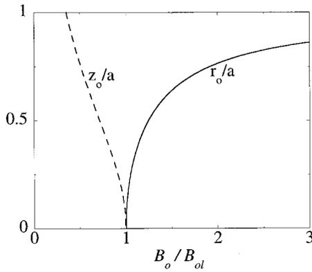
FIG. 3.  $r$  and  $z$  location of the field null as the ratio of the solenoidal to loop field is varied. No  $B_\theta$  field is applied.
