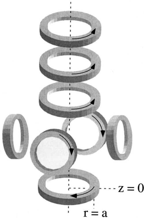
FIG. 6. Schematic of the magnetic coils for a TOP Penning trap.
