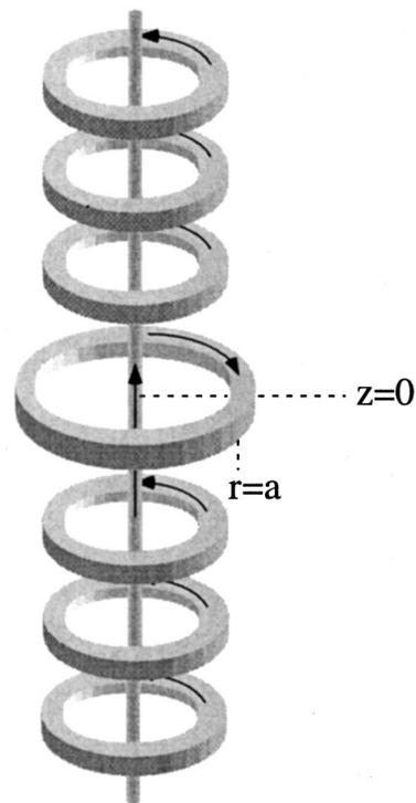
FIG. 2. Magnetic coil configuration of a cylindrically symmetric minimum- $B$  Penning trap.
