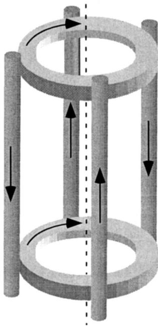
FIG. 1. Magnetic coil configuration of an Ioffe–Pritchard neutral atom trap. Arrows show the direction of currents.
