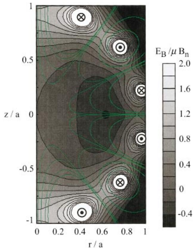
FIG. 9. (Color) The Boltzmann potential from an approximate  $n=6$  multipole, created by 6 current loops. Gray contours are contours of constant  $E_B / \mu B_n$ , for maximum well depth ( $\alpha=0.85$  chosen such that  $E_B=0$  at  $r=a$ ). Green lines are magnetic field lines.
