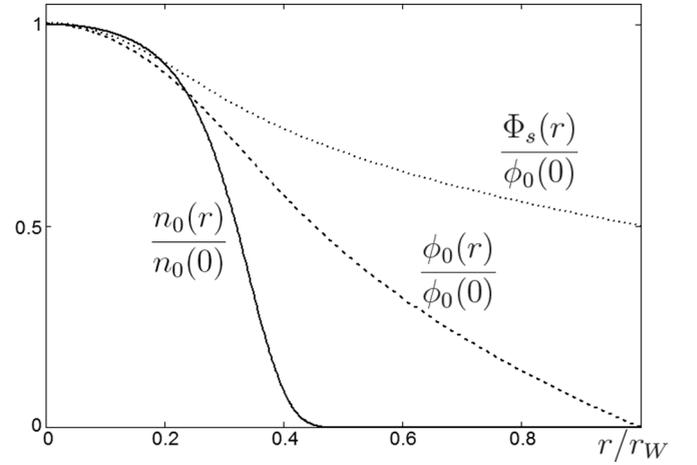
FIG. 1. The solid, dashed, and dotted curves show the radial dependence of the scaled density, potential, and squeeze voltage, respectively [i.e.,  $n_0(r)/n_0(0)$ ,  $\phi_0(r)/\phi_0(0)$ , and  $\Phi_s(r)/\phi_0(0)$ ].
