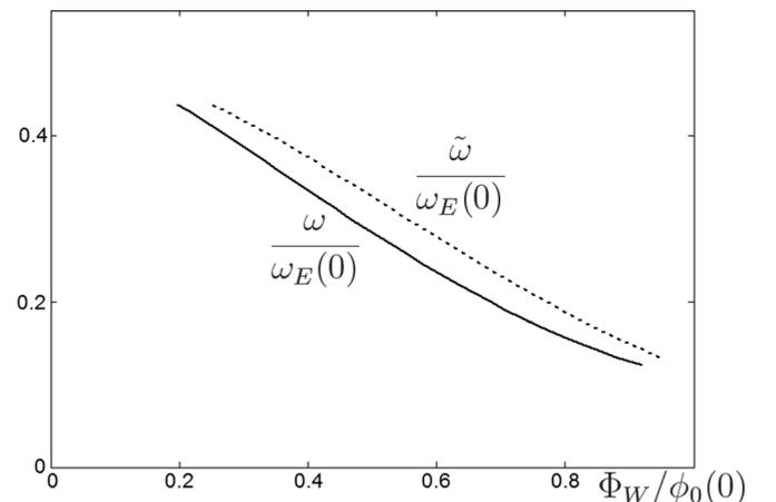
FIG. 2. The scaled frequencies  $\omega/\omega_E(0)$  and  $\tilde{\omega}/\omega_E(0)$  are plotted versus the scaled squeeze voltage applied at the wall,  $\Phi_W/\phi_0(0)$ . The ratio of the Debye length to the wall radius is taken to be  $\lambda_D(0)/r_W = 0.057$ , which corresponds to  $T = 1$  eV in the experiments of Ref. 1.
