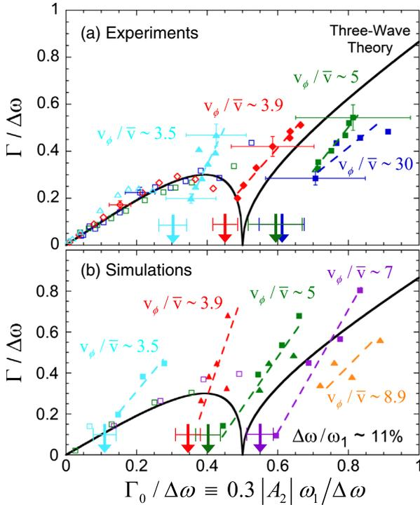
FIG. 4. Measurements (a) and simulations (b) of OCR and exponential growth rates at different plasma temperatures. The reduction in the instability threshold (arrows) at lower  $v_\phi/\bar{v}$  contradicts fluid theories.
