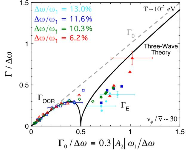
FIG. 3. Measurements of the oscillatory coupling (open symbols) and exponential growth (closed symbols) rates normalized to  $\Delta\omega$  versus the scaled pump wave amplitude for various  $\Delta\omega/\omega_1$ . Solid black curve is three-wave theory.
