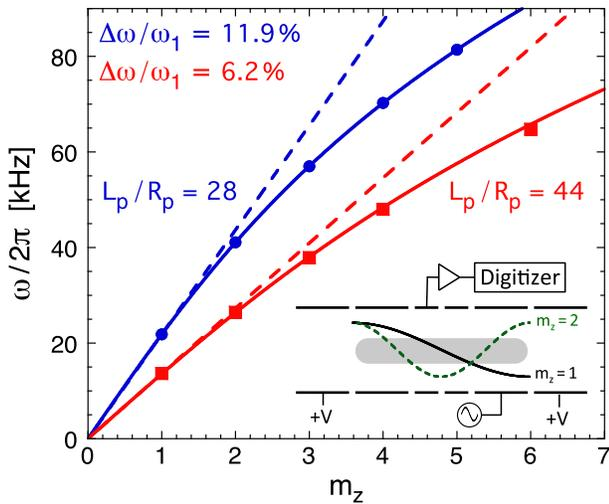
FIG. 1. Measured frequencies of standing TG waves (symbols) for two different plasma lengths on very cold plasmas with  $T \sim 10^{-3}$  eV and  $v_\phi/\bar{v} \sim 90$ . Solid curves are one parameter fits to Eq. (1).
