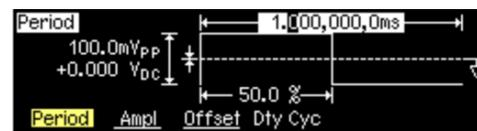
7. You can specify a signal by its amplitude and offset, or by setting its **Hi Level** (maximum) and **Lo Level** (minimum) values. See Chapter 1 in the *User's Guide* for further information.
