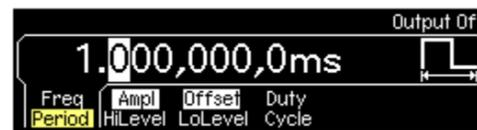
6. In Graph Mode, the softkeys work just as in Menu Mode, except that only one label is displayed for each key. You can still toggle between related parameters such as **Freq** and **Period**:
